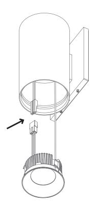
**9.** Insert the trim and attached module into the cylinder. Press until fully seated into cylinder.
