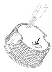
**2.** Line up your trim onto the module and push the trim until the tension clips snap into place.
