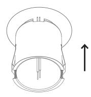
5. Push the flanges on the spring clips out, making sure that the notches on the spring clip snap into place with the T-shaped cutout in the housing.
