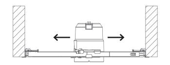
**4.** Lock the horizontal positioning by fastening both bar hanger screws (factory installed).
