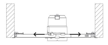
**3.** Adjust the horizontal position of the housing by sliding it along the bar hangers. Locate the center according to the desired fixture location.
