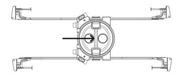
2. Install the bar hanger ends into the joists by nailing in four nails (factory installed) at the end of the bar hangers.
