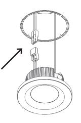
**5.** Place the module into the housing and push the trim up until flush with ceiling.
