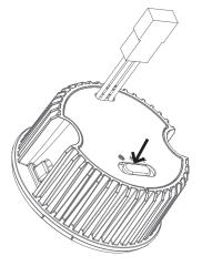
**2.** Line up your trim onto the module and push the trim until the tension clips snap into place.
