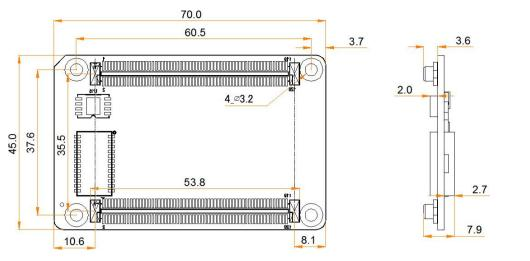
Tolerance: ±0.1 Unit: mm
