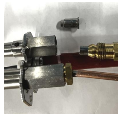
Figure 9.3 – Cleaning pilot orifice
