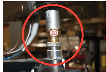
Figure 9.1 – Locating orifice for cleaning
