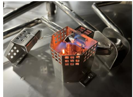
Figure 9.2 – Pilot flame coverage of thermocouple.
