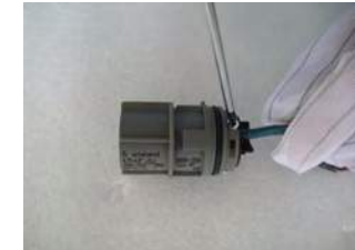
▲ Figure 4.16 Connect Wires to the Terminal
