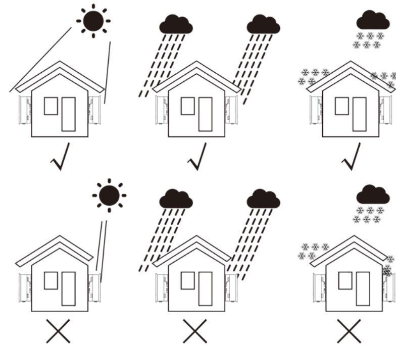
Figure 4.1 Recommended Installation locations
