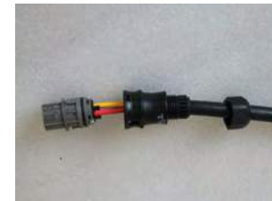
▲ Figure 4.16 Connect Wires to the Terminal
