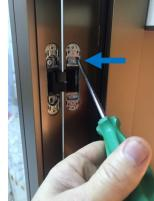
${\it 3. Tighten\, the\, loosened\, screws.} \, Repeat \, this \, process \, for \, the \, other \, hinges.$
