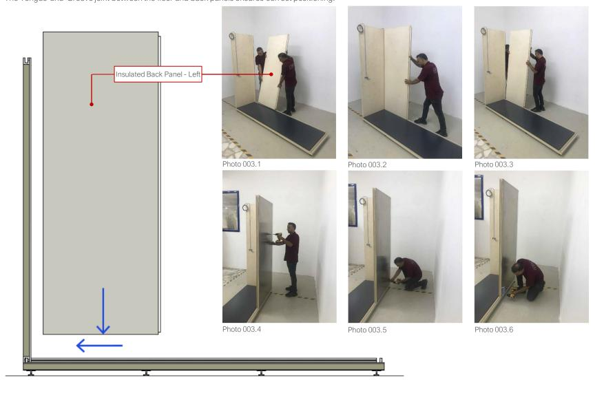
Position as illustrated with arrows in the drawing and securely screw the Insulated Back Panel - Middle using the designated screw holes. The Tongue-and-Groove joint between the floor and back panels ensures correct positioning.
