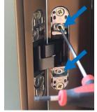
2b. If the adjustment plate of the hinge is slid outward by means of a screwdriver, the door moves away from the cabinet body, reducing the pressure on the door gaskets.
