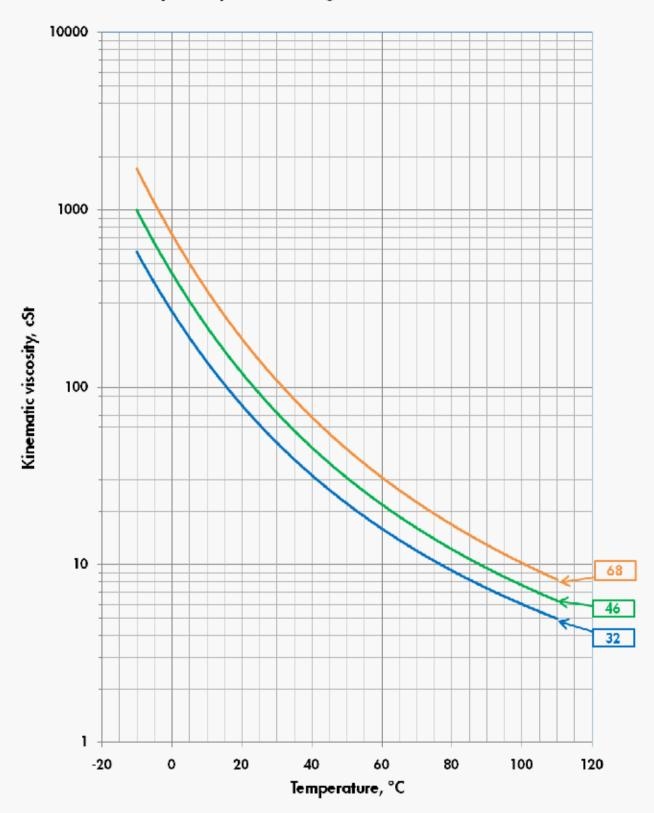
Viscosity - Temperature Diagram for Shell Corena S4 R
