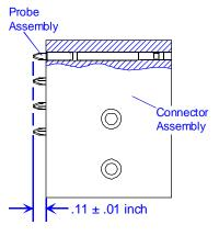
4. Carefully insert the new Probe Assembly, UIC part number 46223001, into the Connector Assembly. Push the probe assembly in until the outside cylinder is flush with the edge of the connector assembly.
