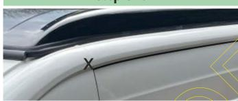
From the designated start point X as shown in the photo This is the front start point for the main rail on all variants of the VW Crafter/Mercedes Sprinter/Man TGE 13 L4 & L5
