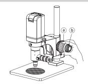
Place Object on the bottom plate and rotate
