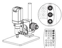
Assembling Completed.\*Use Remote Control or Software to adjust brightness.
