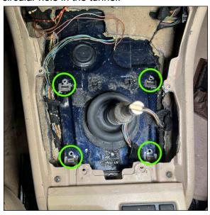
The clips should have a fair bit of resistance sliding into the chassis. If the clips are loose, bend the ears of the clip down until they are snug with the transmission tunnel.
