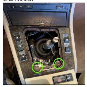
Pull out the center storage cubby and remove the 4 screws in the panel. Disconnect the connectors behind the panel.
