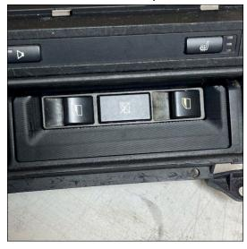
Re-attach the electrical connections to the driver's side window switch.
