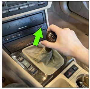
Remove the shift boot by squeezing the sides.
