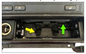
Clearance the center console panel using the supplied template. Match the corner cutout with the center console protrusion.
