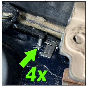
Slide the Handbrake mounting plate over the studs and install the 4x nuts onto the studs. Mounting Nut - (6.2 ft\*Ib, 8.5 N\*m)
