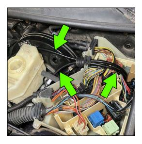
Route the lines along the dash below the steering column and to the center console area.
