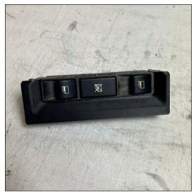
Install the switch and adapter into the center console panel.
