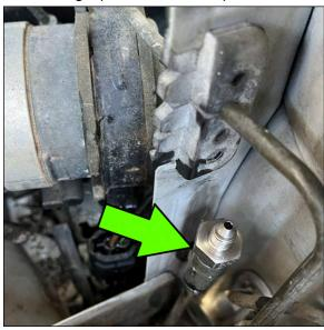
Attach line labeled "return" through the strut tower grommet and to the fitting on the ABS line. Be sure that the return line is not contacting the braided line. *Return Line - (8.3 Ft\*lb, 11.3 N\*m)*
