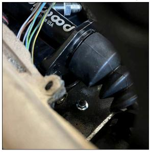
Install the cylinder bolts through the cylinder and into the base. Cylinder Bolt - (18 ft\*Ib, 25 N\*m)
