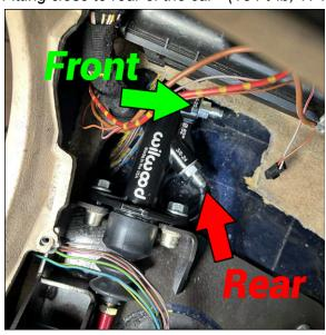
Attach line labeled "feed" to the handbrake fitting closer to the front of the car. Attach line labeled "return" to the handbrake fitting closer to the rear of the car. Feed Line - (8.3 Ft\*lb, 11.3 N\*m)
