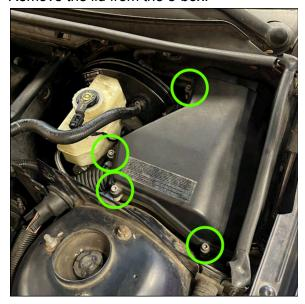
Remove the air filter panel, plastic guard, and brake booster vacuum hose.
