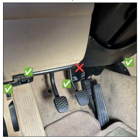
Bend the tabs on the 12v plug to clear the handbrake cylinder.
