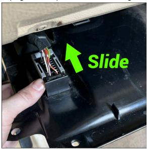
Remove the firewall plate from the e-box.
