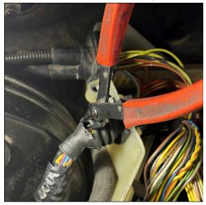
Pass the 2x brake lines through the wire loom grommet hole.
