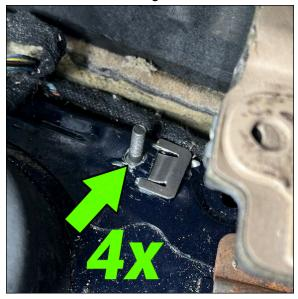
Slide the Handbrake mounting plate over the studs and install the 4x nuts onto the studs. Mounting Nut - (6.2 ft\*lb, 8.5 N\*m)
