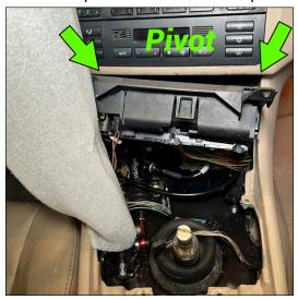
Pull the handle back and pivot the center console panel down into position.
