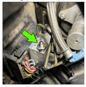
Attach line labeled "return" to the fitting on the ABS block. Be sure that the return line is not contacting the braided line next to it.
