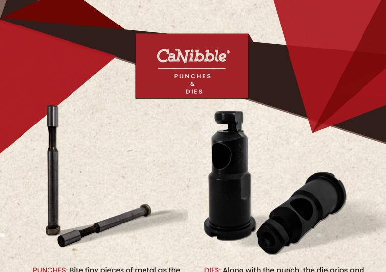
PUNCHES: Bite tiny pieces of metal as the CaNibble cuts, they are made with premium quality high speed steel. Punches are consumable and will dull with use. Each punch offers approximately 550 feet of cutting life.
