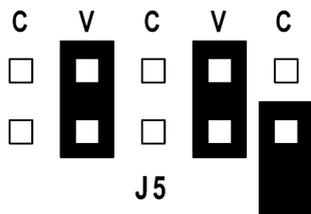
Note that the spare jumper has been fitted to a spare **Current/Voltage Output** jumper pin. This is a safe place to keep it, in case the **proCHEM-R** needs to be reset to current output in the future.
