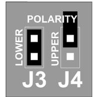
To reverse the action of the Upper Limit, and have two Limits that activate the High and Low LED's and relays when the reading drops **below** the Limits, set the J3 and J4 jumpers as shown.
