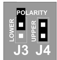
To re-set the action of the Upper and Lower limits to factory defaults, set the J3 and J4 jumpers as shown
