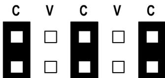
The jumper settings for 0 to 1V DC output are:
