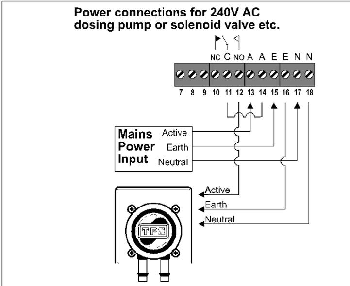
**Power connections for low powered dosing pump or solenoid valve etc.**
