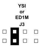
(b) When the miniCHEM-DO<sub>2</sub> is set to ppM readout and the samples have a high salinity, there may not be enough adjustment available with the SPAN control to calibrate the unit. If this is the case, set the YSI or ED1M (J3) jumper to the following setting...
