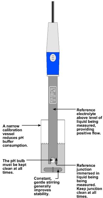
**DO NOT** place the sensor(s) directly into the buffer bottle. Discard the used buffer after use.
