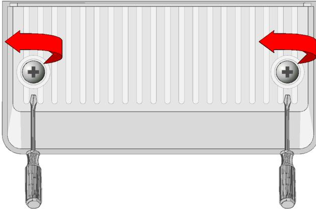
2. Raise the fold out stand (so it is out of the way) and then fully loosen both screws. It is not necessary to pull the screws all the way out. Lift off the battery cover.
