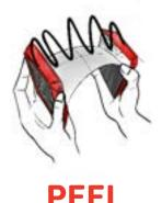
Remove the protective liner under your CellAED® by continuing to separate the two halves. This will expose the integrated gel pads and extend the connecting cable.
