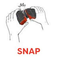
Power CellAED® by snapping in half along perforated centre line. This will automatically start the audio instructions guiding you on what to do, every step of the way.
