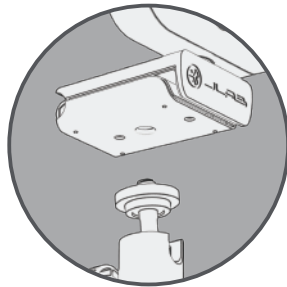
Threaded attachment for tripod-type mounts
