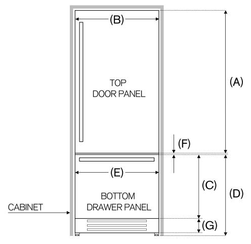
**NOTE**: These specifications assume a standard toe kick height of 4". For different toe kick heights, adjust C accordingly. C must be between 21 1/2" and 25 3/4".
