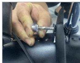
7. Put the screw into the lamp's mounting bracket, install it on the fender mounting bracket
