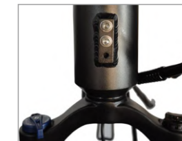
16. There are 3 holes in total, please select the top 2 holes for installation, as shown in the figure
