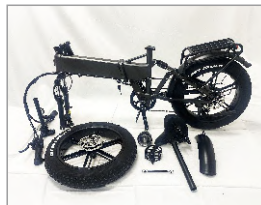
1. As shown in the figure, the front wheels of the bicycle you receive are separated from the bicycle body.
