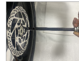
10. Remove the screw on the end of the axle rod and insert it into the front wheel bearing
