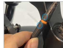
9. Link the light wires, and note that the arrow symbols of the terminals need to correspond to each other
