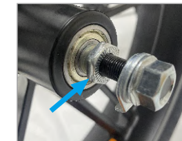
11. As shown in the figure, tighten the nuts marked at both ends of the central shaft
