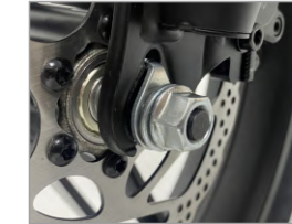
13. Tighten the nuts at both ends of the center shaft as shown
