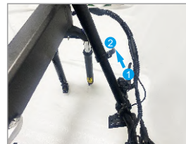
2. Insert the pipe 1 into the riser 2 to the mark on the riser 1, and lock the quick release device.
