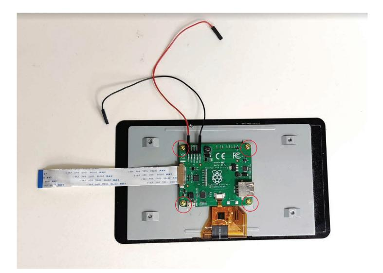
Attach the display to the housing using the green screws as shown below. Feed the white ribbon cable through the slot in the center of the housing. Feed the fan power leads through the hole at the top.
