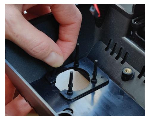
Then pull the rubbers mounts through the fan holes and pull the thin end of the mount until the fan is mounted on the rubber mount as shown below. The fan should only be mounted in the way as shown below.
