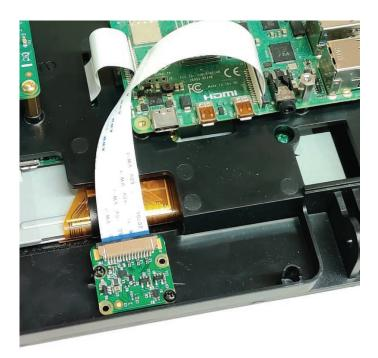
Do not overtighten the screws!
