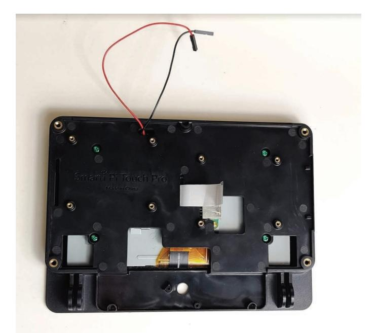
If using the port blocking part, from the back side cut out the desired ports with a utility knife. Two parts are included. One for Pi 2/3 and one for Pi 4.
