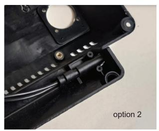
Use the two small black screws to secure the small plastic retaining part to the back cover. This will hold the power cable in the case.
