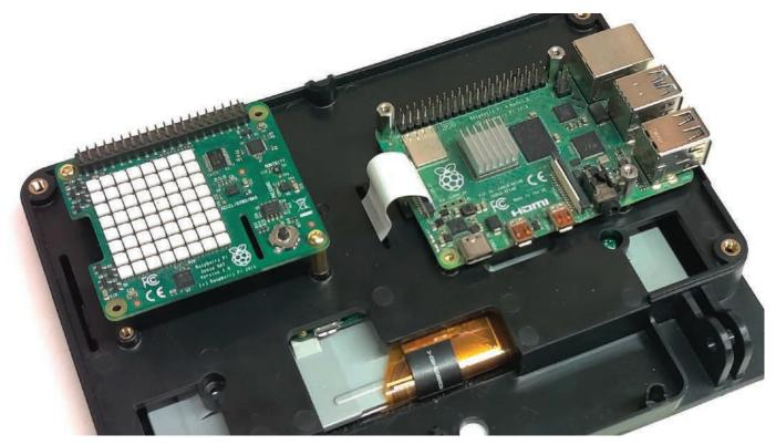
You can choose to mount the Raspberry Pi in the other set of brass inserts if you wish. Although you won't have access to the USB and ethernet ports from the outside. We offer small extension cables in our store that extend USB port access and audio jack access back out to the side of the case when mounting the Pi in this configuration.
