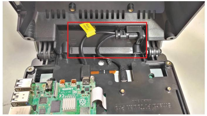
If you are mounting the Raspberry Pi as shown below, you may need to mount the cable input at the farther out position and rotate the connector so that the Raspberry Pi cable lead is positioned closer to the Raspberry Pi as shown below.. This will give you more slack in the cable.
