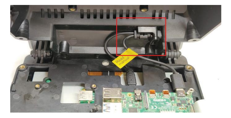
Assemble the back cover to the display housing with the four black screws. The port blocking part should have tabs that fit inside the housing and cover.
