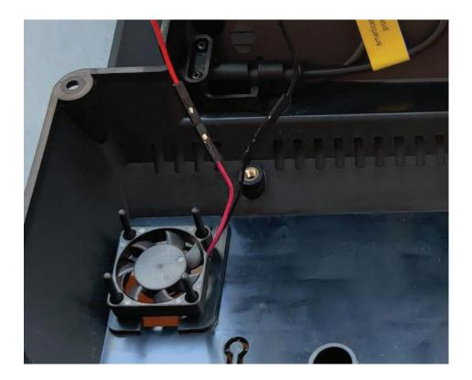
Attach the power cables to the Pi and the display. You may choose to flip the position of the cable input so the power leads are not cossing each other and for more efficient wire routing.
