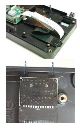
3 Cut out the raised plastic at the edge all the way down to the main plastic surface as shown in the red box to the right.
