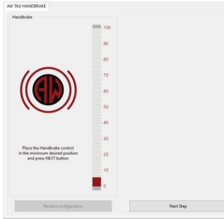
Fig. 12. Calibration Menu – Setting the Minimum Signal Value.
