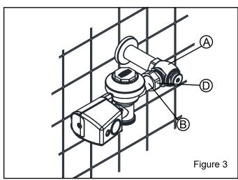
**3.)** Insert the flush valve tailpiece **(B)** into the stop valve **(A)** and hand tighten the lock nut **(D)** to the stop valve. Plumb the entire unit
