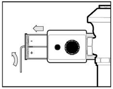
STEP A Use battery compartment wrench STEP B Pull cover off by rotating batto remove battery compartment tray.
