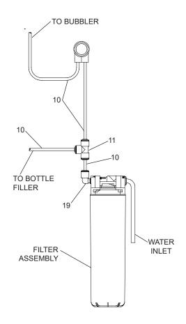
Figure 3 - LZLMSN-EDFPVM214DK Tube Routing
