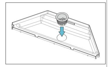
4. Install the O-ring over the strainer threads.
