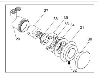
Figure 10 - Bottle Filler Push Button Assembly
