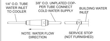
Figure 11 - Water Supply Connections
