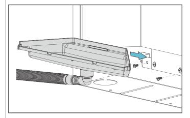
8. Connect the drain adapter into the household waste drain pipe.
