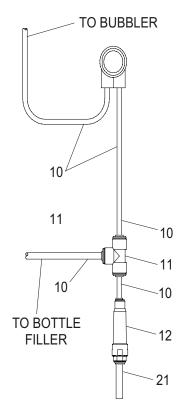
Figure 2 - EZLMSN-EDFPVM214DK Tube Routing
