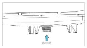
5. Thread the strainer into the drain adapter. Needle-nose pliers can be used to hold the drain adapter from the top while tightening. Ensure that the connection creates a watertight seal. The drain adapter must be facing to the left.
