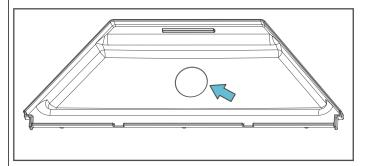
3. Trial fit the strainer. If the strainer does not fit, carefully open the size of the hole. If it fits well, place a small amount of plumbers putty around the lip of the strainer flange and insert it into the hole.
