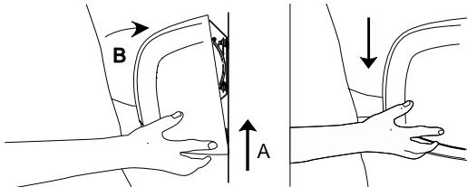
1. Replace cover by positioning top of cover on studs on top of mounting base and tipping bottom of cover toward wall. Push bottom of cover firmly against wall.
