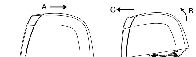
2. To remove cover, place a hand on each side of cover and push up toward top of dryer releasing cover from studs at top of mounting base. Lift cover off mounting base by pulling forward at the bottom and upward at the same time.
