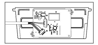
If top cap stiffener piece is installed, remove by simply pulling out. Install endpoint board assembly by sliding inside using rail feature shown below. Ensure it is secured properly.
