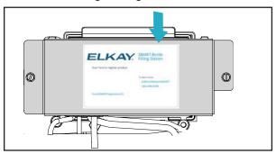
14. Install back bottle filler to the wall mounting plate and refasten using (2) screws making sure gasket is properly placed beneath the bottle filler.
