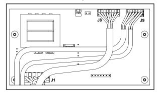
6. Remove (4) T-10 Torx screws to remove control board.
