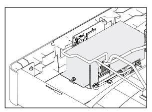
13. Apply plumbSMART registration ID label at desired location. Recommended on cover (shown below) or next to the product label underneath of basin (at step 15). Avoid any location that has the potential for vandalism / damage to registration ID information.
