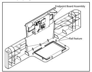
11. Connect endpoint board cable to J7 connector on the main board, as shown below.
