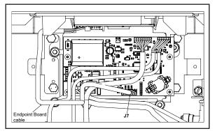
12. Replace the main control board cover. Ensure all the cable are organized to exit from the cable opening as shown and refasten the cover using (2) screws.
