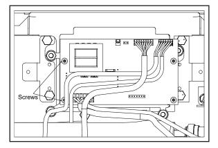
Replace new connected-ready control board and refasten using (4) T-10 Torx screws.
