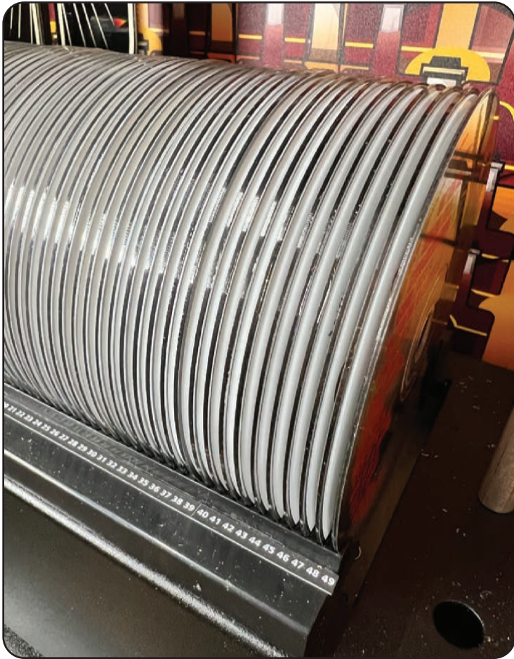
FIG4 : CDs inserted into the mechanism Note the printed side is facing towards the right
