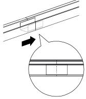
**5.** Now press the second gutter completely over the gutter extension to form a seamless joint
