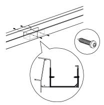
**6.** The gutter connector can now be secured with the short stainless steel screws in the chamber of the gutter and on the front side under the decorative profile. Apply sealant onthe assembly so it is smooth and waterproof!
