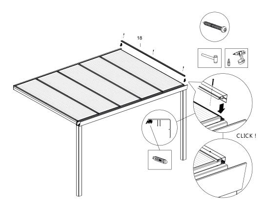
**12.** Now screw a sheet stopper at the gutter end of each middle beam to ensure secure attachment. **Note:** securing the end cover strips comes later.
