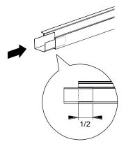
**1.** Clean and degrease the gutter and the gutter extension.
