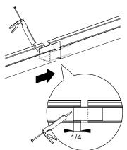
**4.** Insert the second gutter ¼ of the way into the other side of the extenstion and apply sealant on the edge.
