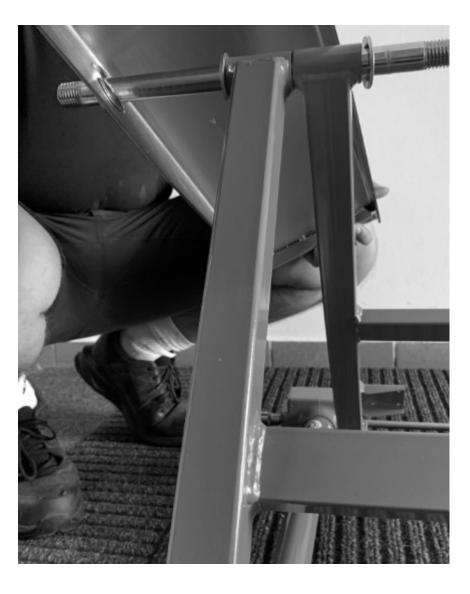
Screw the nut onto both sides of the axis bolt and tighten securely with a 30 mm wrench.
