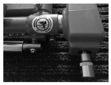
The usage of air/pneumatic/impact tools or tools having shocks. Damage to the lifting gear drive.
