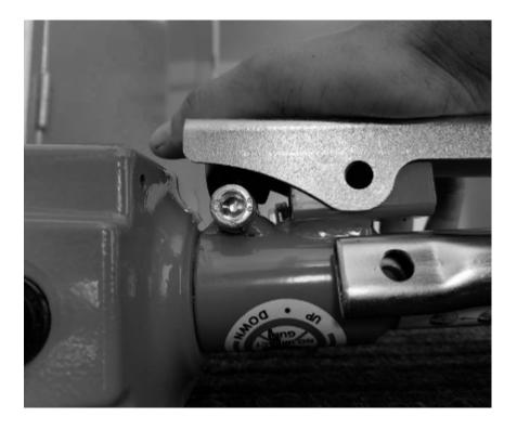
Insert the pin included in the Rails for uneven surfaces accessory through both holes and slide the spacer onto it.
