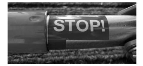
**Exceeding the minimum permitted lower limit.** Risk of damage to the lifting gear drive.
