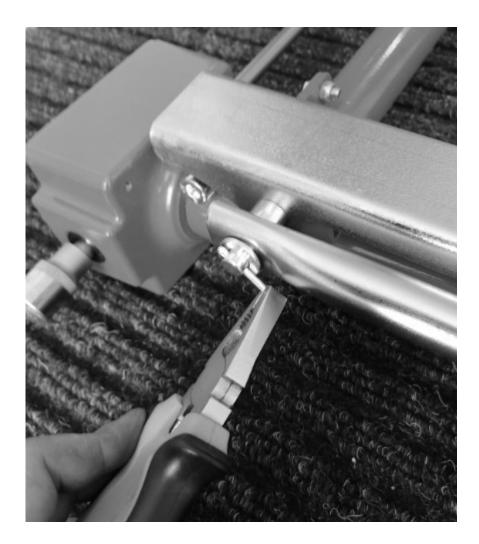
Place one of the rails for uneven surfaces on the lift, ensuring that the holes are accessible from both sides (do not be afraid to push the rail with force).
