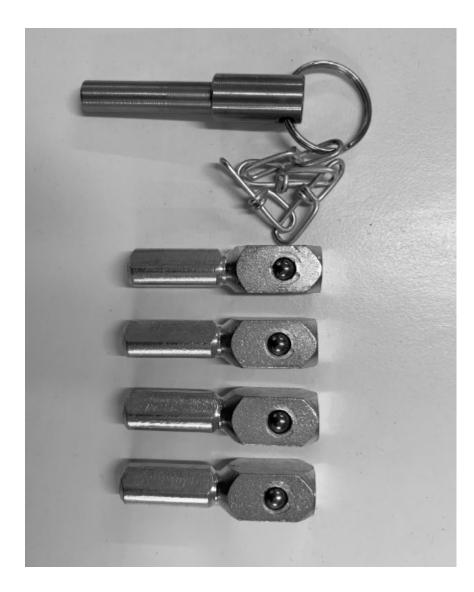
Insert one of the adapters into the drill. The rest of the adapters should be carefully saved.
