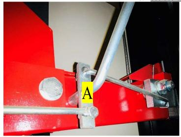
Insert Front Lock Release Lever (A) into the hole on the right front of the lift. Install 1 Jam nut on threaded end once inserted fully.
