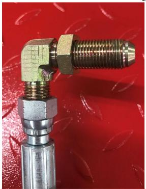
Remove 1 of the 2 nuts from the 90 degree fitting under the runway.
