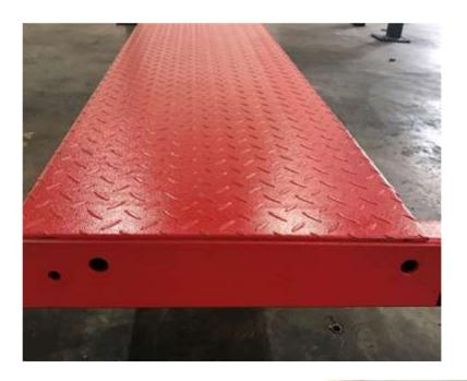
Once both cross beams are sitting in the columns, place runway between the cross rails with lips sitting on top of cross rails. Be sure to leave the smooth edge of the runway facing outwards.
