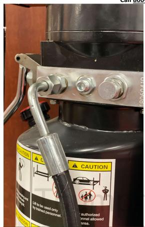
Connect 90° end of hydraulic cable to power unit (Like shown in Picture 1)
