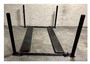
Arrange the 8 major components in a configuration conducive to assembly.
