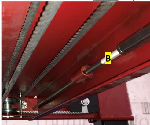
**Insert Rear Lock** Release (B) into the hole on the right Rear of the lift.
