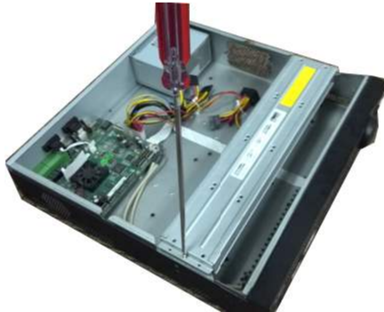
Figure 3-36 Open the top cover
