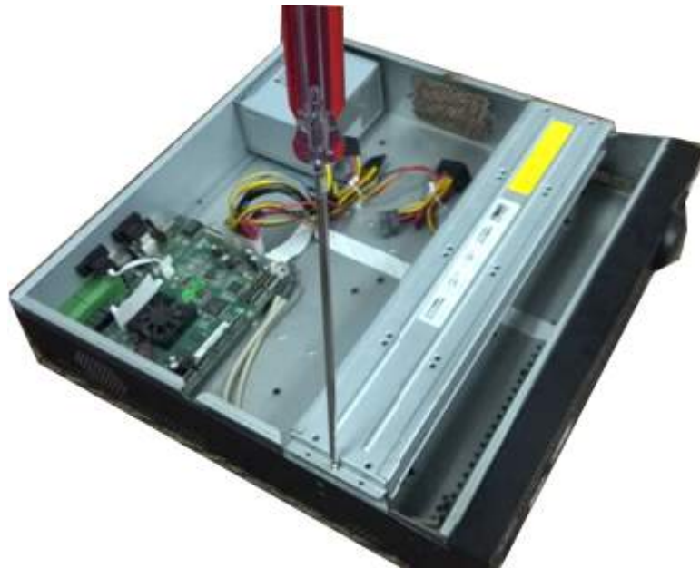
Figure 3-36 Open the top cover
