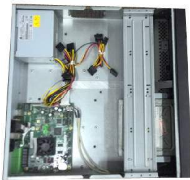
Figure 3-44 Put bracket back
