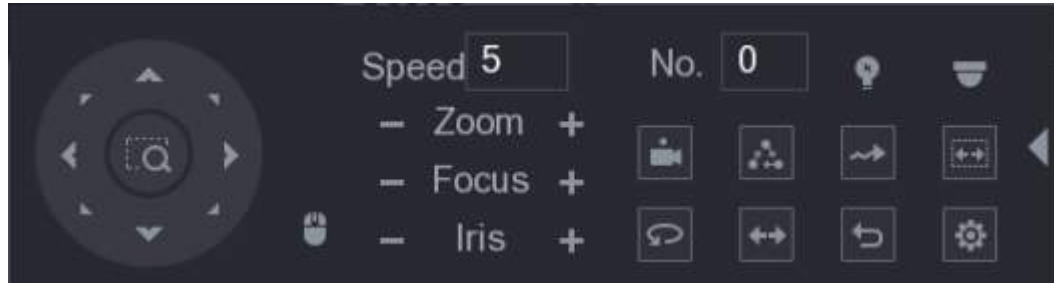
Figure 5-59 Expanded PTZ control panel
