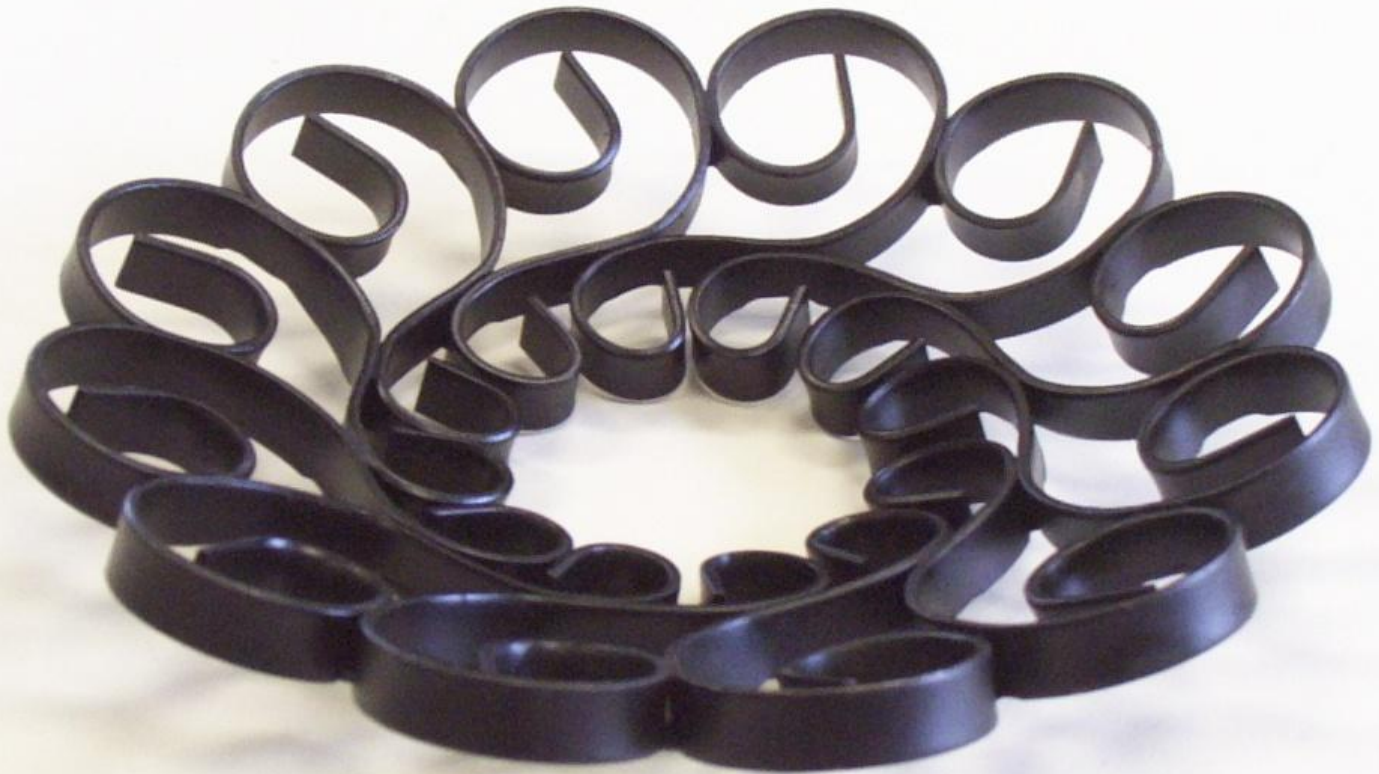
A scroll ring section after being dished.
