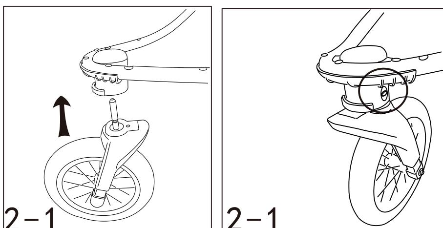
2. Assemble the front wheel: insert the axle of the wheel into the hole TILLA SOUND "CLICK" as picture 2-1.
