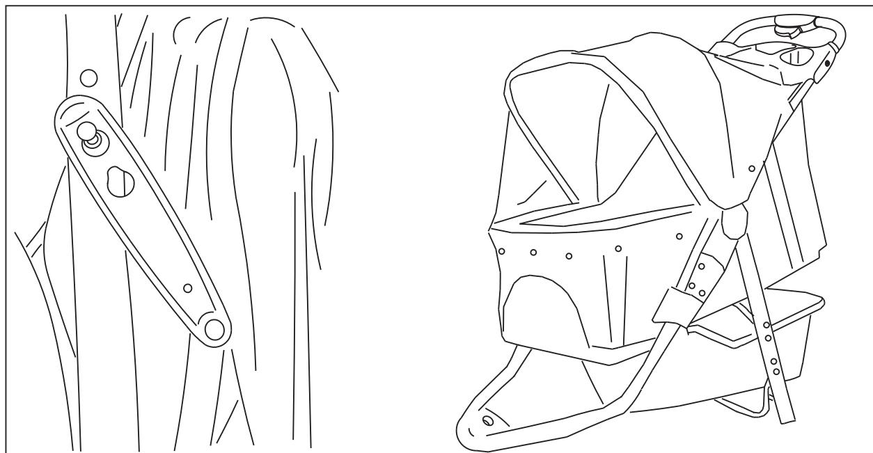
1. To open stroller: release the folding hook as the picture shown, lift the handlebar, unfold the stroller and make sure both joints locked.
