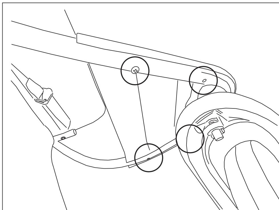
4. To attach footboard: attach footboard position to bottom and tighten screws.
