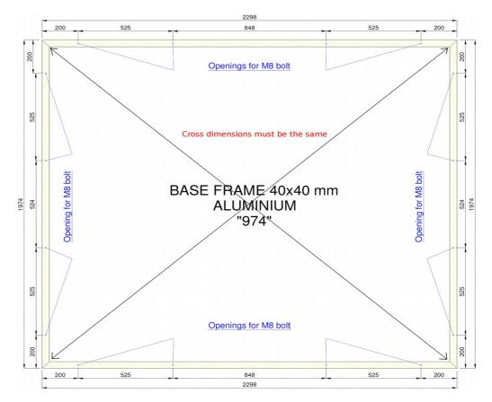
After aluminium base frame is anchored, the aluminium or wooden frame is screwed on top of the aluminium frame.
