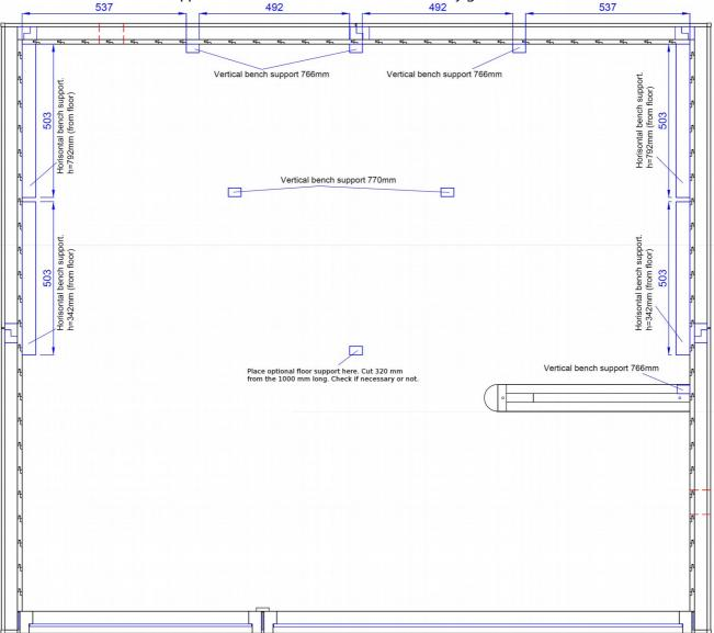
\* Place vertical 766 mm supports so that their bottom is at the same level as wall paneling bottom. \* Attach 2 horizontal 503 mm supports on the side walls so that they are 4 mm from back wall and their
