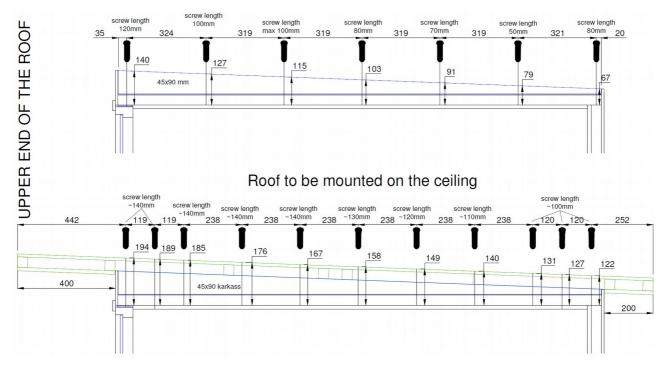
Roof in 2 parts. Lift up the roof parts. Screw them in place with right length screws to the rafters.
