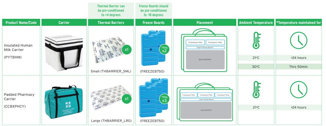
\*Study by TuV GmbH. Freeze Boards preconditioned to -18°C for 24 hours. Thermal Barrier preconditioned to 4 degrees. For more information please contact us.
