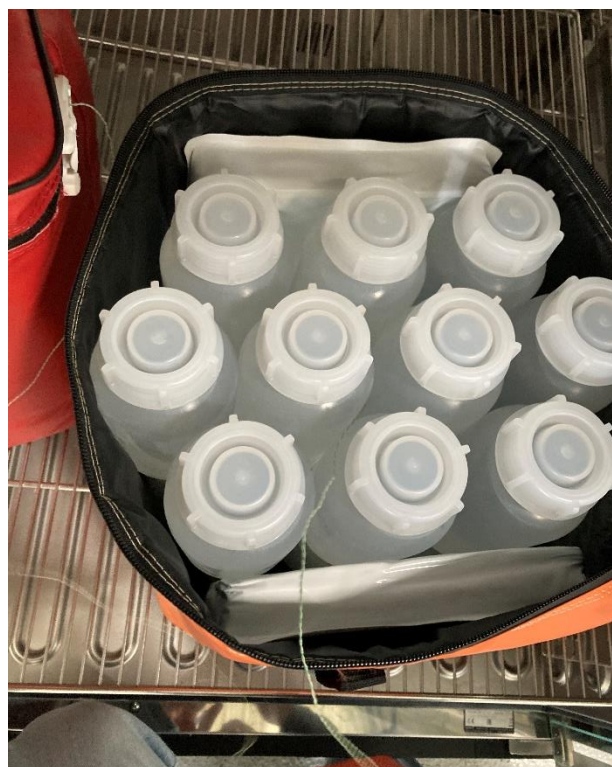
Figure 7 – Placement of the plastic bottles and the ICECATCHs in the test sample "Thermal Bag"
