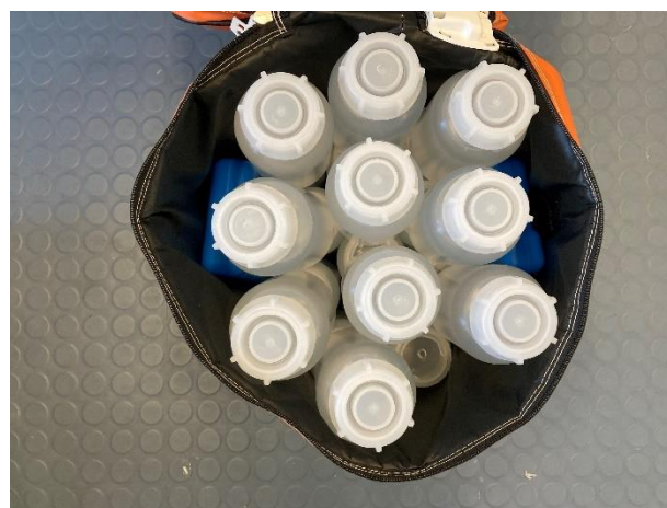
Figure 11 – Placement of the plastic bottles and the Freeze Boards in the test sample "Thermal Bag"
