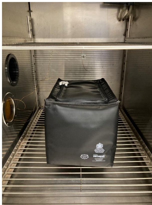
Figure 18 – Test sample "Ice Bag" in the Temperature test chamber before the test
