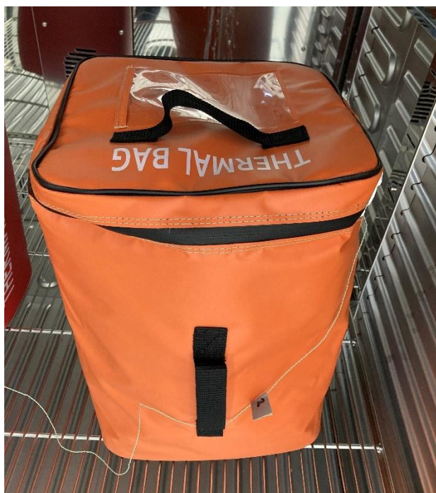
Figure 12 – Test sample “Thermal Bag” in the Temperature test chamber before the test
