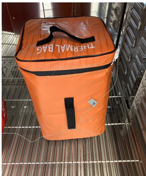
Figure 8 – Test sample "Thermal Bag" in the Temperature test chamber before the test
