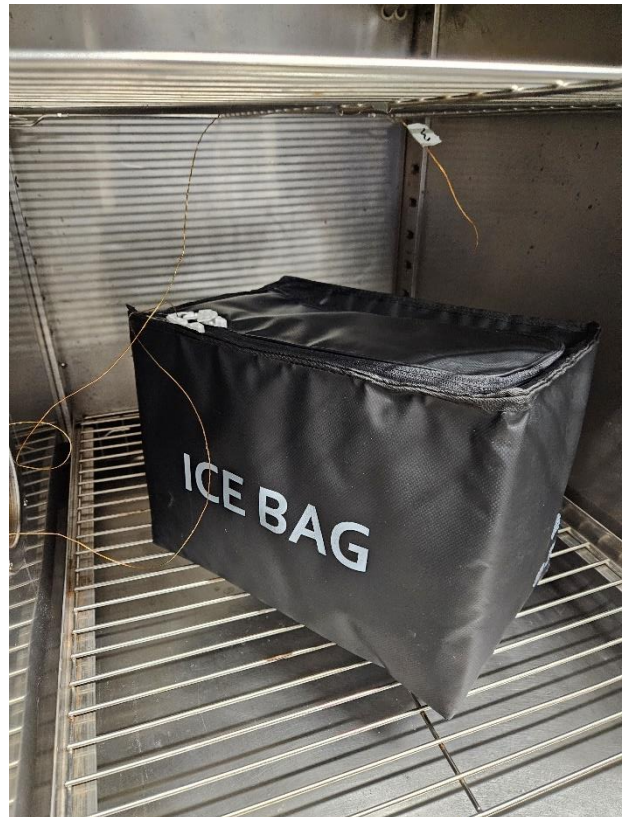
Figure 15 – Test sample "Ice Bag" in the Temperature test chamber before the test
