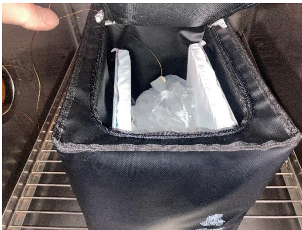
Figure 14 – Placement of the temperature sensor, ice cube and the ICECATCHs in the test sample "Ice Bag"
