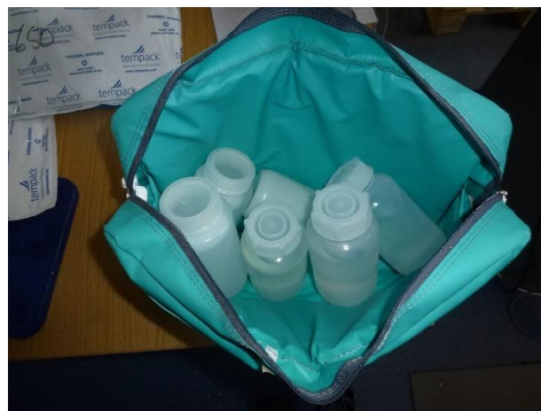
32. VFT6999FRDG_T2 after drop test opened, no damages
