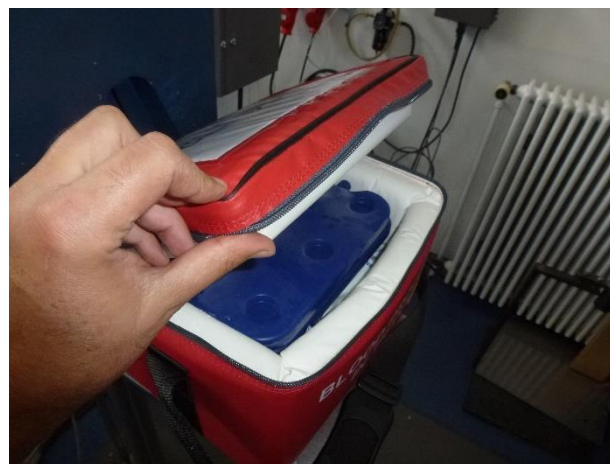
24. BLTD1 after drop test opened, no damages
