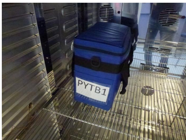
3. Loaded PYTB1 in Temperature chamber
