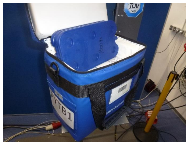
18. PYTB1 after drop test opened, no damages
