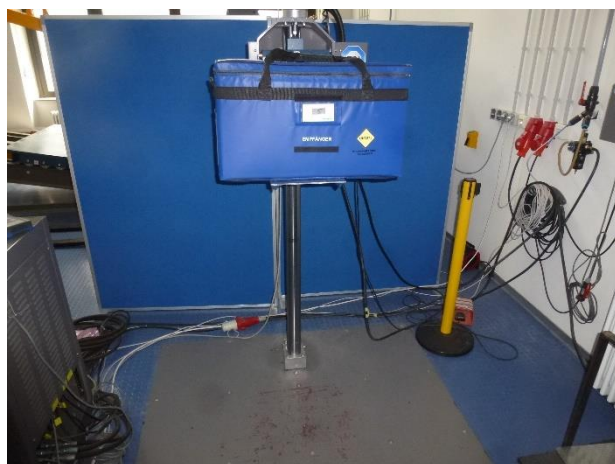
21. PYTB3 before drop test
