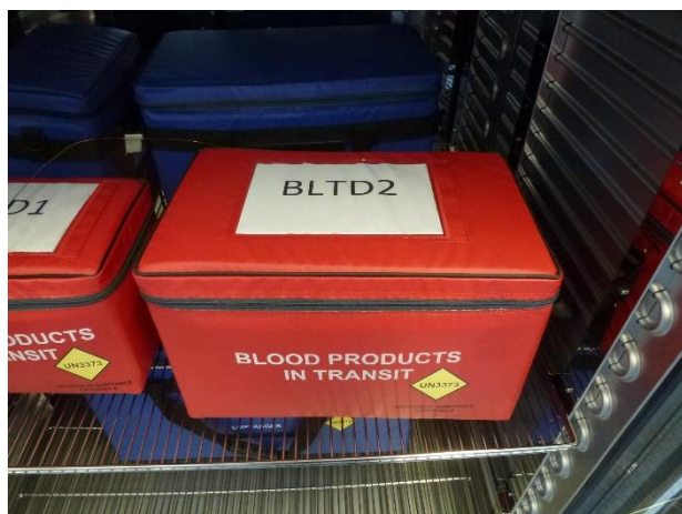
11. Loaded BLTD2 in Temperature chamber
