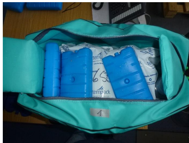
30. CCBX PHCY after drop test opened, no damages
