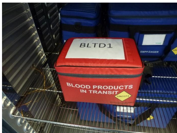
9. Loaded BLTD1 in Temperature chamber
