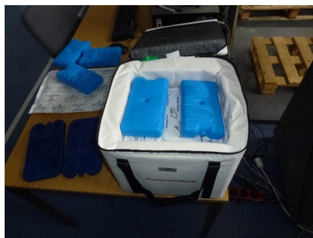
28. PYBHM after drop test opened, no damages
