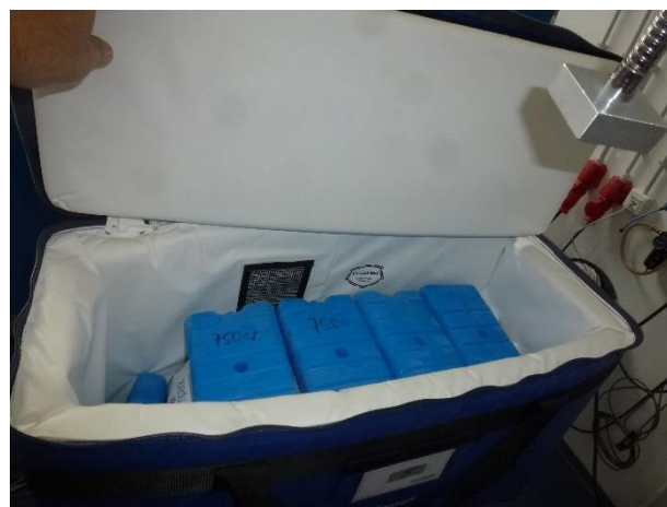
22. PYTB3 after drop test opened, no damages
