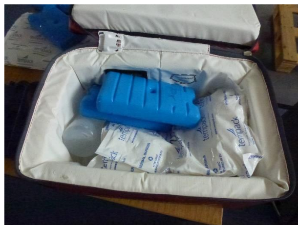
26. BLTD2 after drop test opened, no damages
