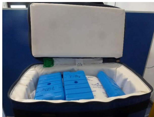
20. PYTB2 after drop test opened, no damages
