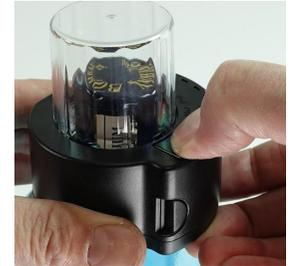
**2** Now press the release button with your left thumb. This should release the Tag from the bottle.
