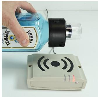
Simply hover the Tag above the Deactivator. The Tag will beep and at this point the Tag is deactivated and is safe to remove.
