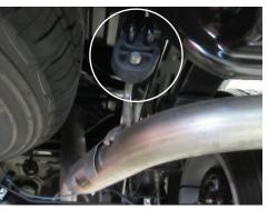
3. Detach the final hanger from the rubber insulator, then remove the OEM exhaust.
