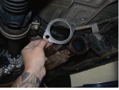
5. Install the provided exhaust gasket.
