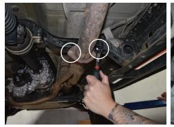
1. Remove the two OEM bolts securing the OEM exhaust.
