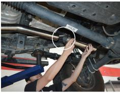
the front extension pipe to the front pipe. Secure using the provided 76mm clamps
