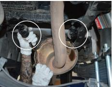
2. Detach the three muffler hangers from the rubber insulators.
