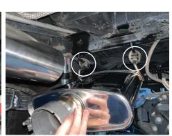
8. DOUBLE CAB LONG BEDS ONLY: Attach 9. Insert the muffler hangers into the rubber insulators.
