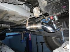
11. Secure the HT-Rear pipe to the muffler section using the 76mm clamps. Once complete, ensure all bolts and clamps are properly secured.
