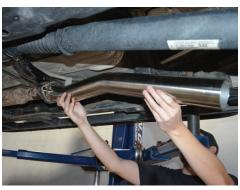
6. Attach the Injen front pipe to the OEM exhaust pipe.
