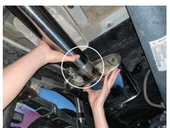
10. Secure the muffler section to the front pipe with the provided 76mm clamps.
