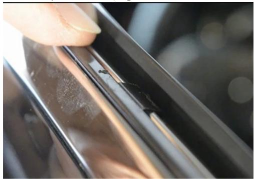
8. Make sure adhesive backing is hanging from below the visor because you'll be pulling the backing from under the visor.
