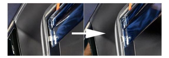
Optional step: Peel off and stick the optional protective film between the bracket and door frame.
