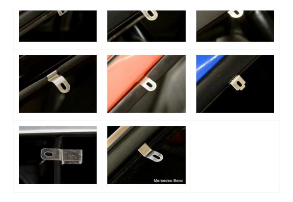
After insertion of the clips, raise and lower the window several times to seat the door glass run channel.
