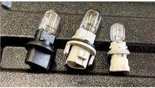
Disconnect all bulb holders from factory harness. Remove factory bulbs from the larger sockets as these will be used to connect to new harness.
