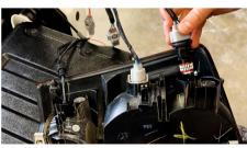
Install brake light sockets. Twist switchback bulb into the reverse light socket. Tuck wiring out of the way and firmly push the tail light to snap into place. Tighten bolts. Repeat for other side.
