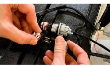
Connect factory bulb holders to the new brake splitter harness. Plug the red LED bulbs into the brake light sockets. These bulbs are dual polarity so orientation should not matter.
