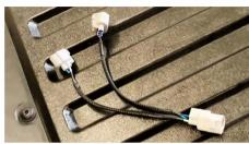
Connect brake splitter harness to the TRIANGLE shaped factory plug.
