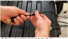
7. Connect switchback bulb to the 3 pin waterproof plug. Tighten nut fully to maintain seal.
