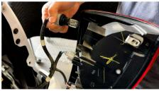
Remove all three bulb sockets from tail light by turning counter clockwise.
