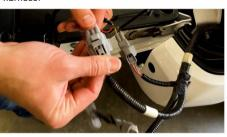
Connect other harness to both of the remaining plugs. The reverse light plug may be difficult to install if pins are bent. Inspect and straighten with flat head screwdriver if needed.
