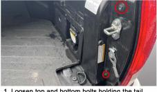
Loosen top and bottom bolts holding the tail lights. The middle bolt does not need to be loosened. Pull the tail light straight back to remove from truck.
