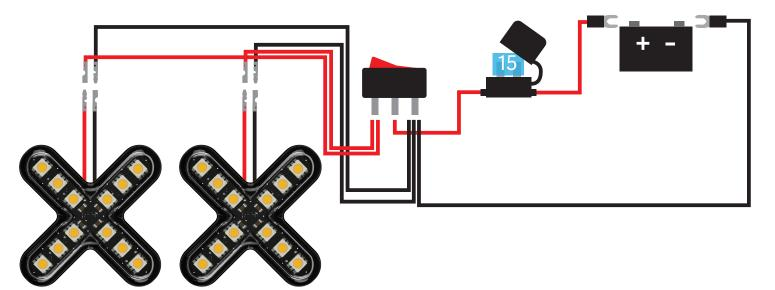
Determine how many ROX lights you are wiring, this will determine the wire gauge and fuse size for inline fuses. For example a standard 14 AWG wire is limited to around 15 amps. Make sure not to overload your wiring.
