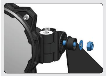
Safely install the Light Bar by aligning the M8 Hardware on the End Mounts to the Vehicle Mounts. (The ambidextrous design of the mounts allow for the threads to be installed in either direction.)
