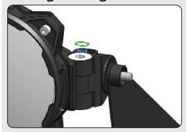
Set the final level & pitch of the Light bar: 1) Tighten the M8 Horizontal Mounting Hardware, allowing the Light Bar to center itself. 2) Torque the M6 Adjustment Screws to 100 in/lbs to lock Light Bar into position.
