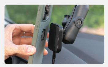
The **Mount Head** magnetically connects to the back of your phone. Once connected, confirm phone is charging via phone screen.
